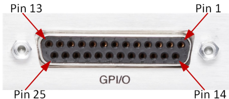
Figure 41: GPI/O Connector Pinout - Rear Panel View
